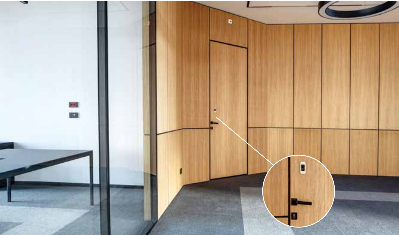
PANEL WOODEN DOOR made of sandwich panel with thickness of 78 mm with veneer structure with metal insert part, wooden panels and insulation. The frame is massive wood with a thickness of 78 mm. Leaf folds it is aligned on the door frame. There is an opportunity for decorative cladding.
