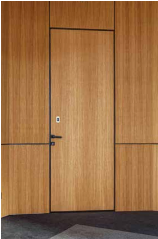
PANEL WOODEN DOOR made of sandwich panel with thickness of 78 mm with veneer structure with metal insert part, wooden panels and insulation. The frame is massive wood with a thickness of 78 mm. Leaf folds it is aligned on the door frame. There is an opportunity for decorative cladding.
