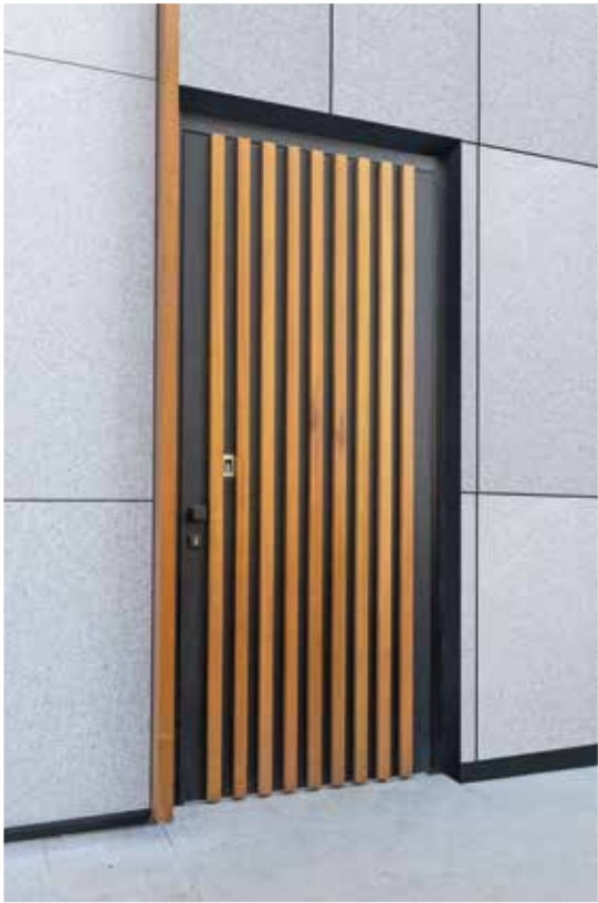
PANEL WOODEN DOOR made of sandwich panel with thickness of 78 mm with veneer structure with metal insert part, wooden panels and insulation. The frame is massive wood with a thickness of 78 mm. Leaf folds it is aligned on the door frame. There is an opportunity for decorative cladding.
